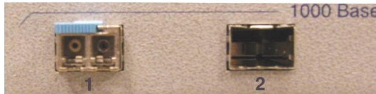
Figure 2.25: Inserted SFP Transceiver in GbE Port 1 (Receive to the left, Transmit to the Right)
