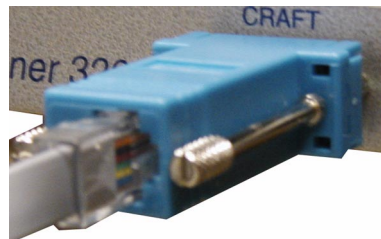
Figure 2.17: Connected Serial Cable
